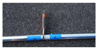
**STEP 3** - A sleeve insert is in one of the pieces which is slotted to allow compression
