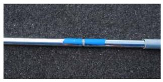
**STEP 5** - Remove the vice grips from the sleeve and then stand the upright on end and tap the end on a solid surface until the two pieces are joined together
